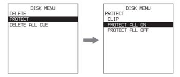
To display the protect operation menu, select PROTECT in the Disk menu and press the ⇒ (OUT) button. In the protect operation menu, select PROTECT ALL ON or CLIP and press the SET button. All clips or individual clips are protected.
